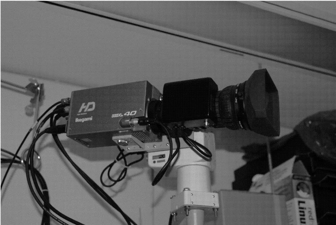
Figure 21: Ikegami HDL-40 camera with Funjinon motorized HD lens and Funjinon Pan&Tilt system
