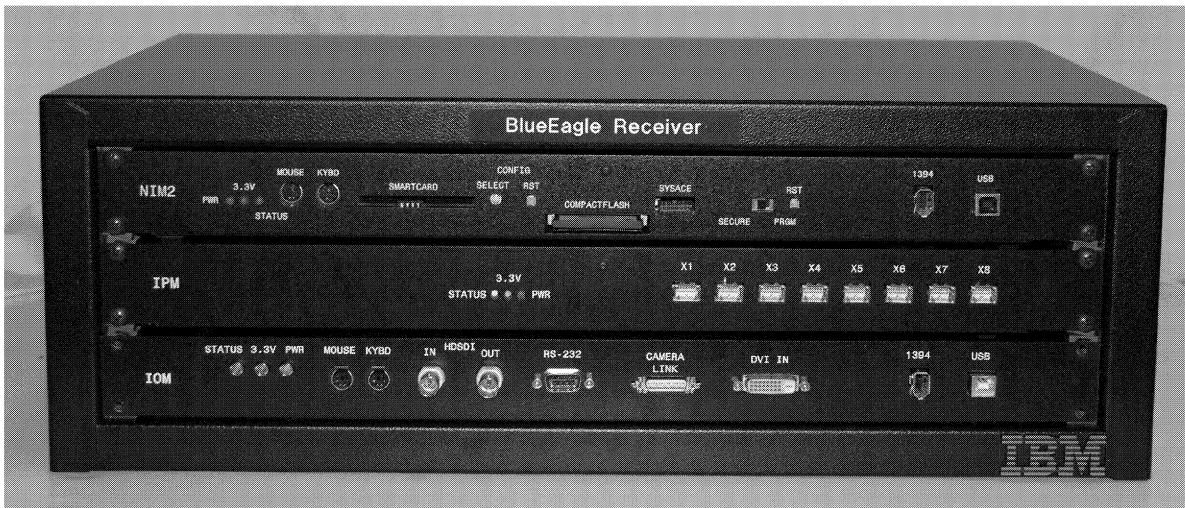
Figure 20: Fully packaged “BlueEagle” receiver system unit using identical hardware modules as in the transmitter system unit but programmed differently to accommodate functionality
