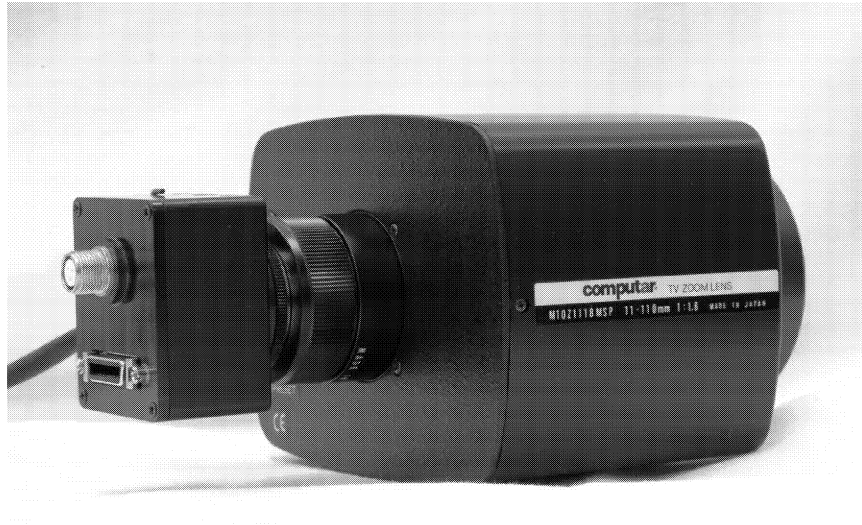
Figure 22: SI-1920HD-RGB Camera Mounted on Computar H10Z1118MSP Motorized 2/3" Lens
