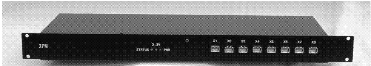
Figure 12: Front view of IPM 19"-rackmountable 1U module with the eight auxiliary high speed interfaces and status LEDs in the front
