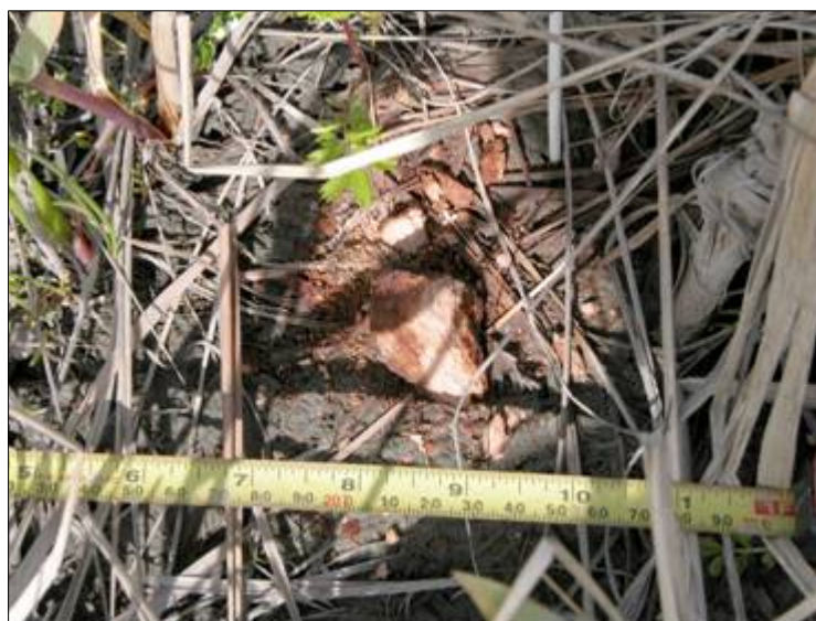
Figure 10. HE particle recovered from the 5-m zone outside a low-order impact area.
