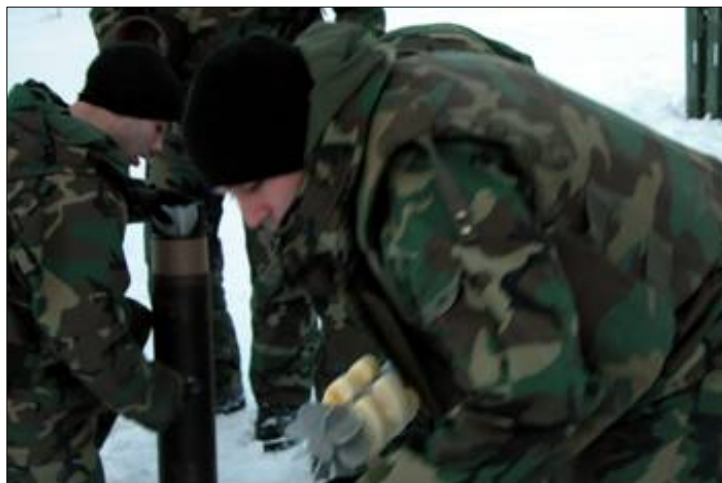
Figure 4. Mortar round with propellant charges on the tail assembly.
