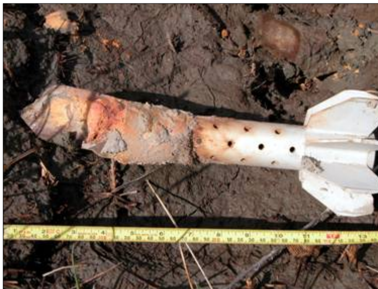
Figure 9. Tail assembly and explosive debris from a low-order 120-mm HE detonation.
