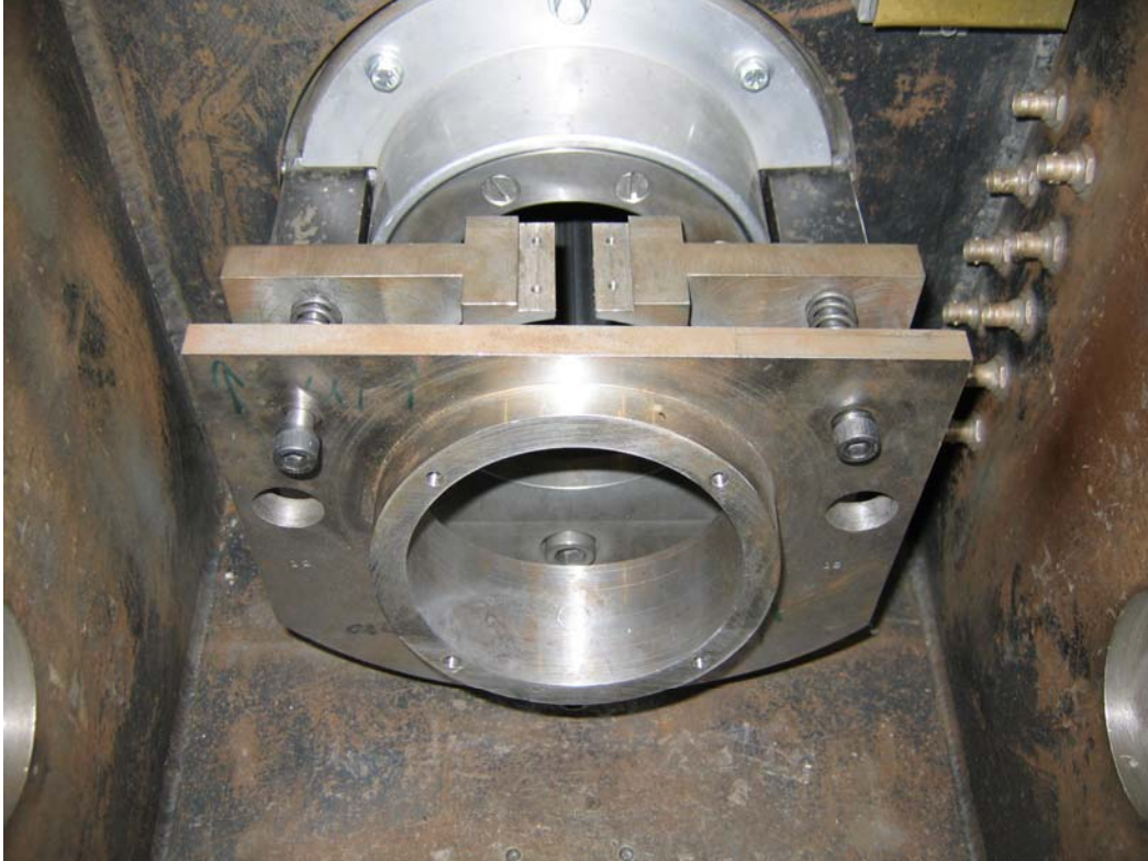
Figure 6. Target mounting plate and tension mounting bolts.
