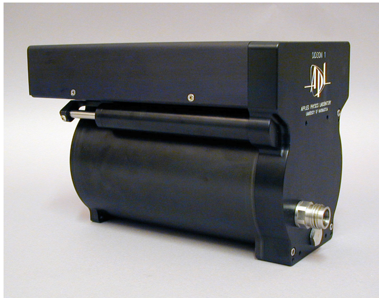
Figure 1. The Dual-frequency IDentification SONar (DIDSON)
