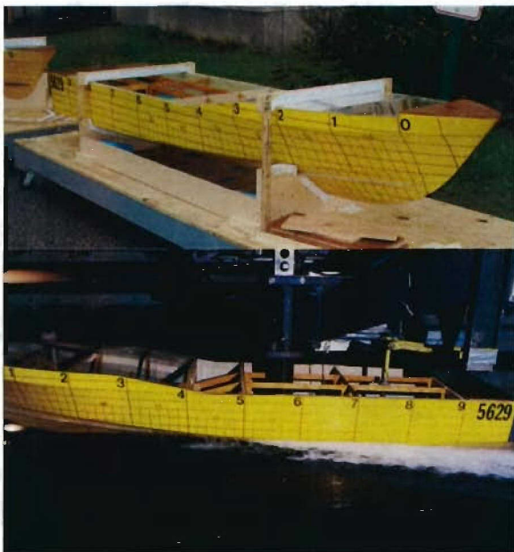
Figure 4. Model 5629 Dry and at 298lbs, 43%, 25.47 Knots
