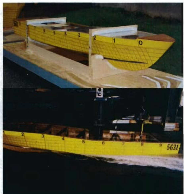
Figure 6. Model 5631 Dry and at 298lbs, 43%, 25.47 Knots
