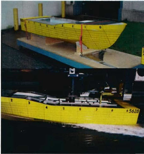
Figure 3. Model 5628 Dry and at 298lbs, 43%, 25.47 Knots
