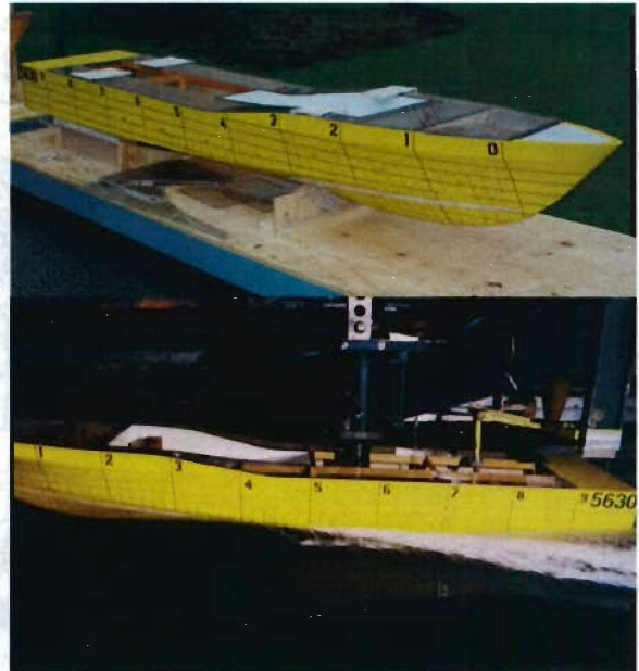
Figure 5. Model 5630 Dry and at 298lbs, 43%, 25.47 Knots
