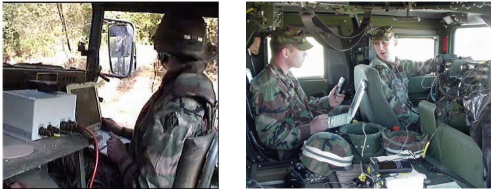
Figure 3. Sensor box installed in HMMWVs
