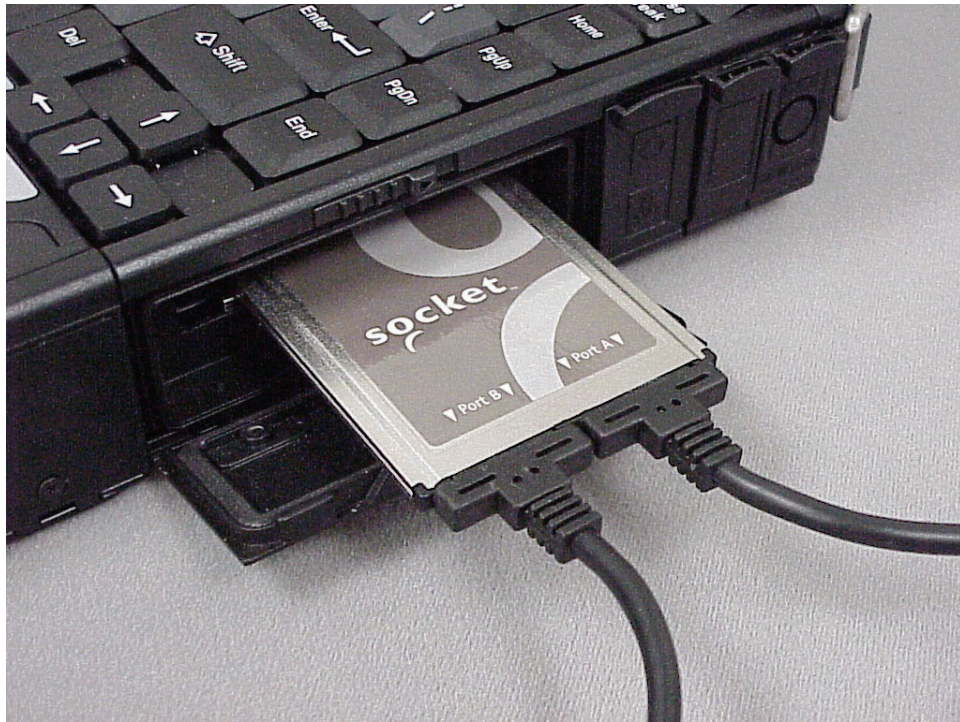
Figure 7. PCMCIA card partially inserted
