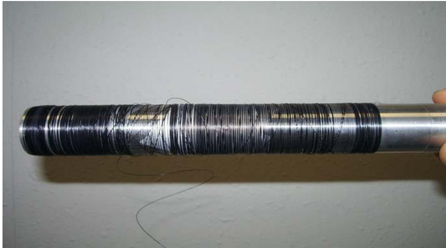
Figure 8: The produced continuous CNT fibers wound on to the take-up bobbin
