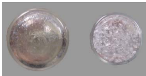
Figure 8: Er:KY 3 F 10 powder in the index matched PFCB polymer (left) and when index is not well matched (right)
