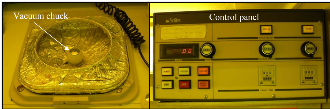
Figure 29. Solitec Photoresist Spinner used to apply PIP material to packaged test dice.
