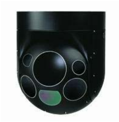
Figure 6. StarSAFIRE III IR detection system employing 640 x 480 indium antimonide mid-IR FPA made by FLIR Systems, Inc [30].
