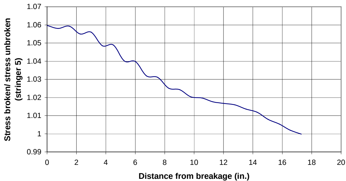
Figure 7 - Relative increase of stress in stringer 5 adjacent to the break in stringer 4.
