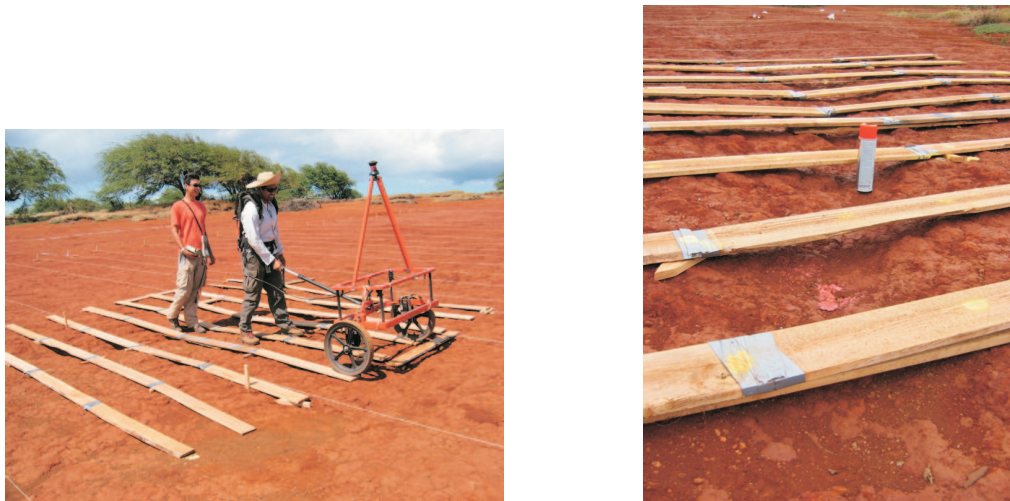
Figure 4.5: Photographs of the detailed grid of planks established to investigate coil orientation within Grid 2E. The photo on the left shows the plank grid during surveying. The photo on the right shows a close up of the rivulet that runs through the grid.
