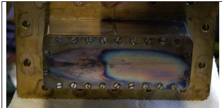
Figure 5. Post-test image of smooth plate showing non-uniform heat marks.
