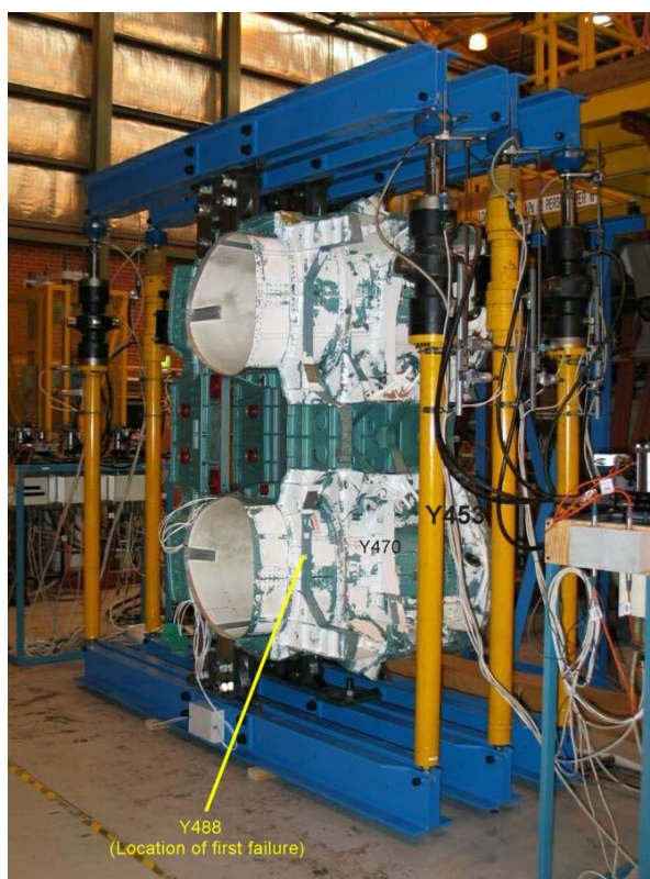
Figure 28: An F/A-18 centre barrel mounted in the FINAL rig (location of first failure highlighted)
