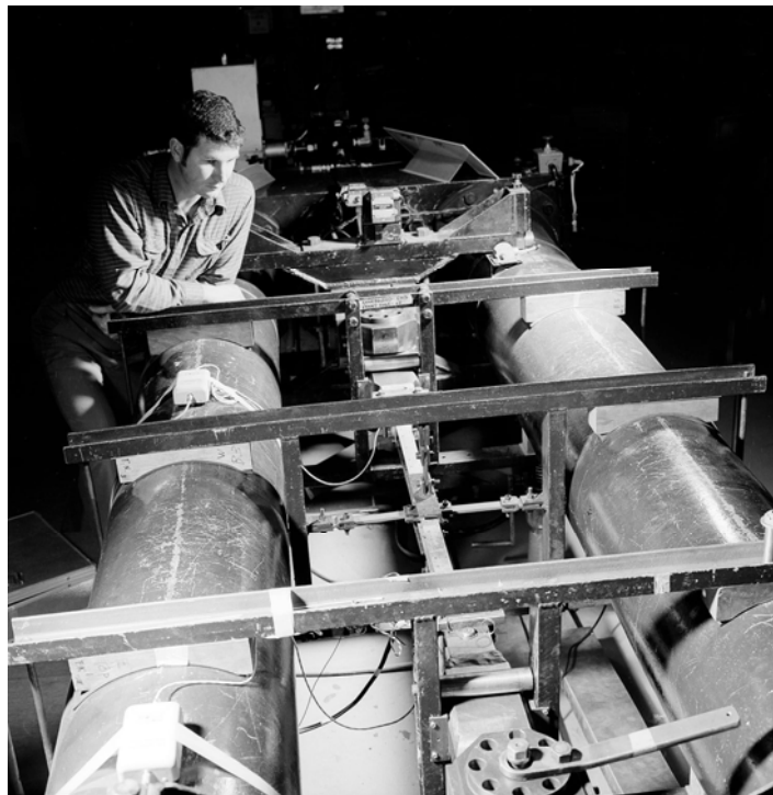
Figure 16: F-111 component test in the Humphries test machine
