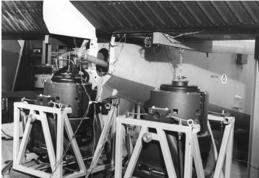
Figure 20: CT4 horizontal tail resonance test rig
