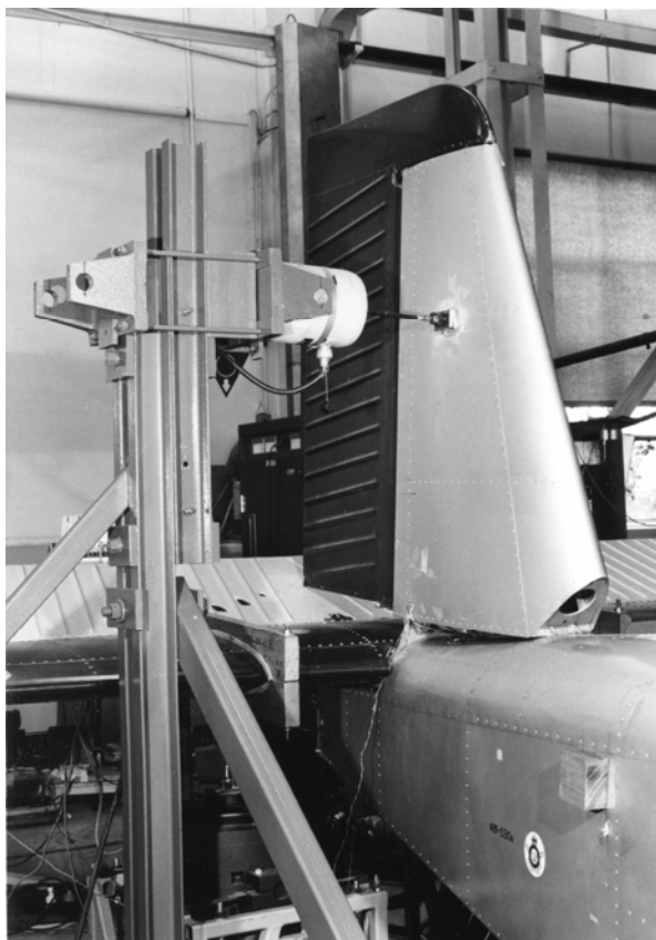
Figure 21: CT4 vertical tail resonance test rig
