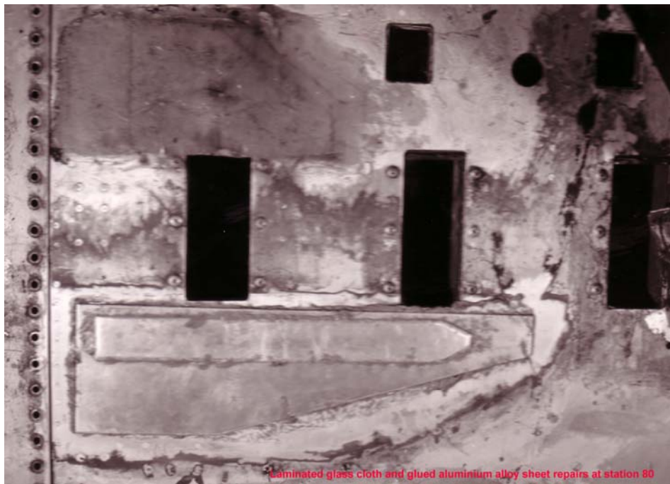
Figure 9: Early DSTO bonded repair on Mustang wing test (laminated glass cloth (above) and bonded metal sheet (below))
