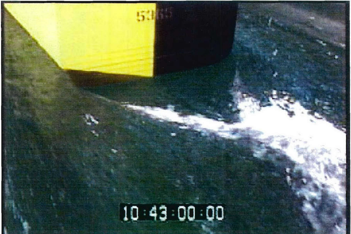
Figure 27: Stern image of Model 5365 during testing at 3.22 m/s (10.58 ft/s), corresponding to 9.3 m/s (30.4 ft/s), or 18.0 knots, full-scale
