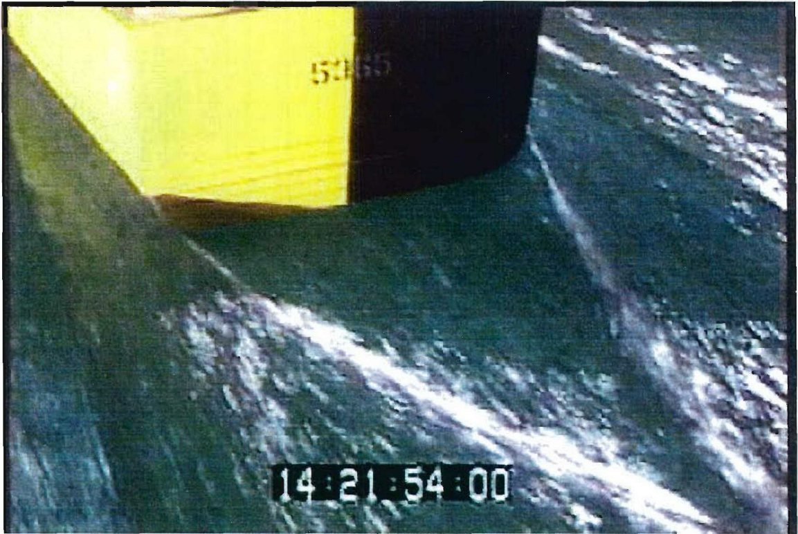
Figure 31: Stern image of Model 5365 during testing at 4.62 m/s (15.16 ft/s), corresponding to 13.3 m/s (43.5 ft/s), or 25.8 knots, full-scale
