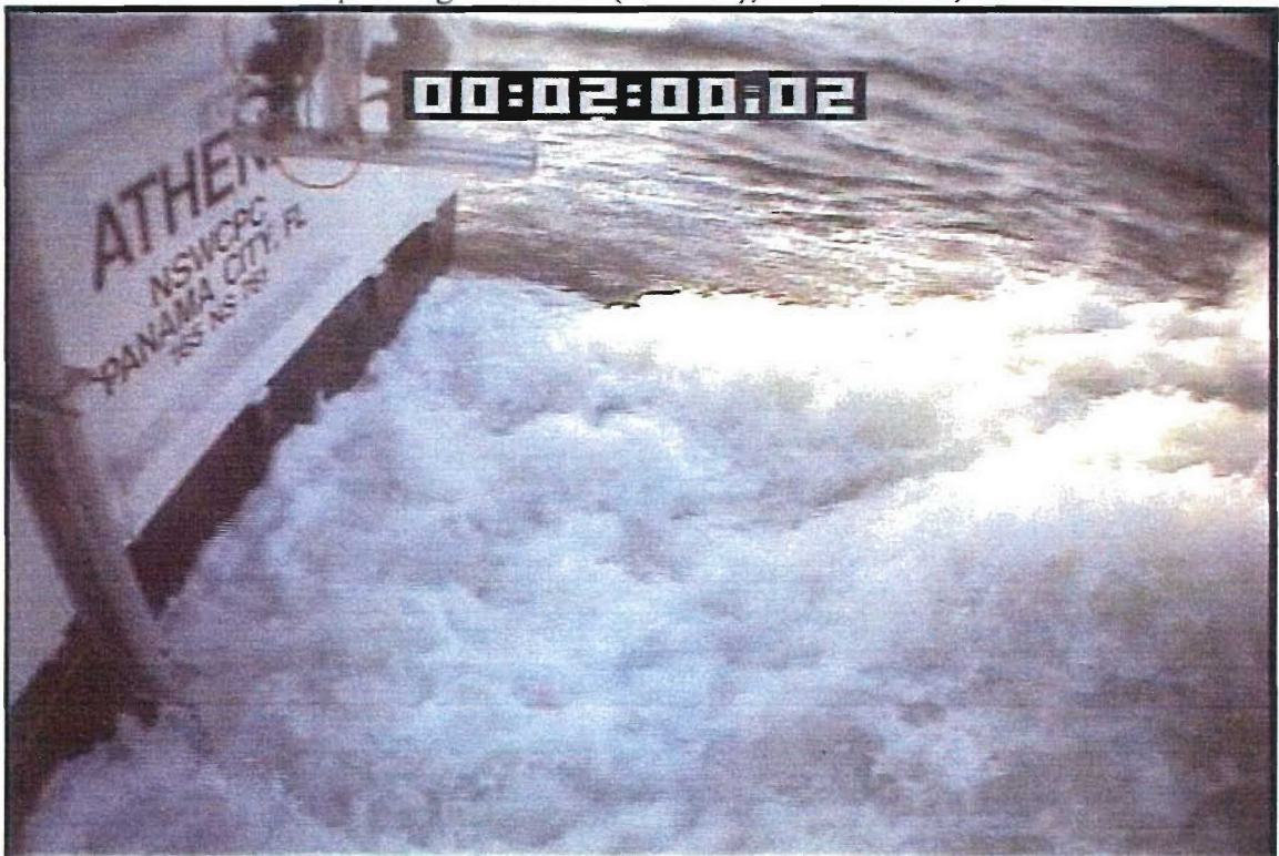
Figure 24: Stern image of full-scale R/V Athena during testing at 5.4 m/s (17.7 ft/s), or 10.5 knots
