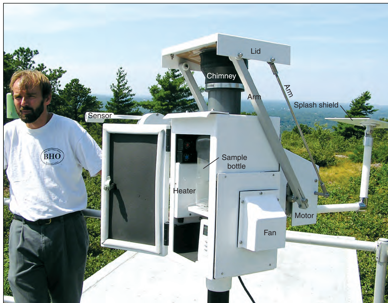
Figure 3. Top-loading N-Con mercury wet-deposition sampler, Blue Hill Observatory, Milton, Mass.
