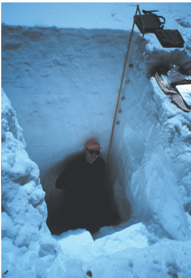
Figure 1. Snowpit face just before sampling the full snowpack.
