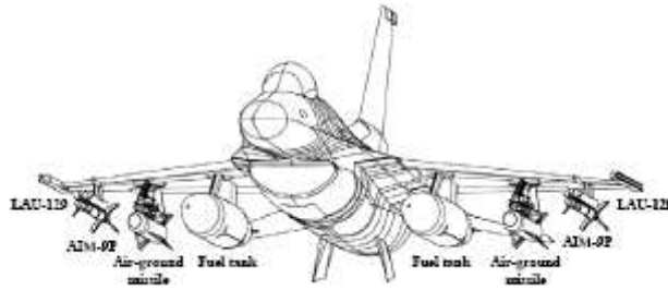
Figure F.1 F-16C Store Configuration
