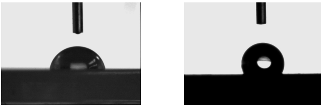
Figure 9: An image of a water droplet on unfilled PVDF (left) is shown next to an image of a water droplet on PVDF blended with ten weight percent fluoroocetyl _8 T _8 .
