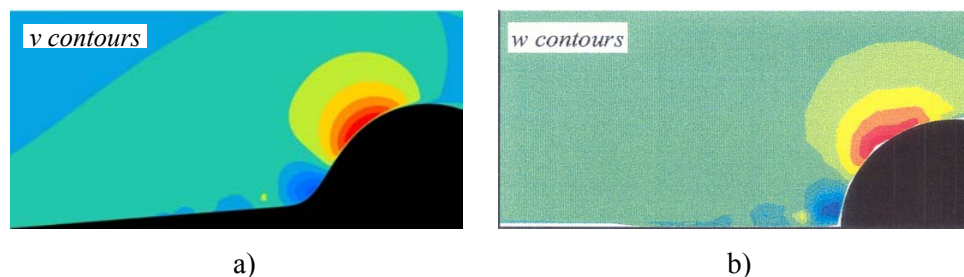
Figure 10. Comparison of time-mean wall-normal velocities between Winkler (1996) experiment and DNS results.
