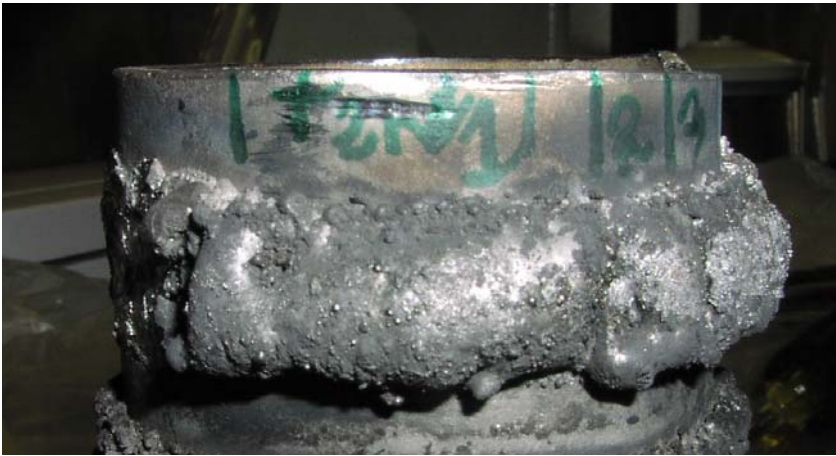
Fig. 9. Continuous beryllium deposit on stainless steel. Deposit height is 6 mm and width is 10mm.
