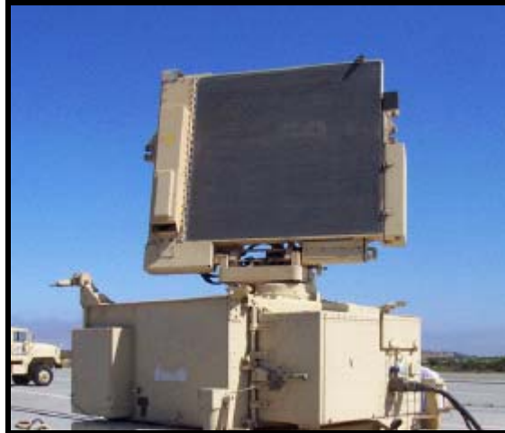
Figure 1. MWR-05XP (Mobile Weather Radar-2005, X-band, Phased Array). Radar shown in its original military operational configuration, mounted on a trailer. ( Back )
