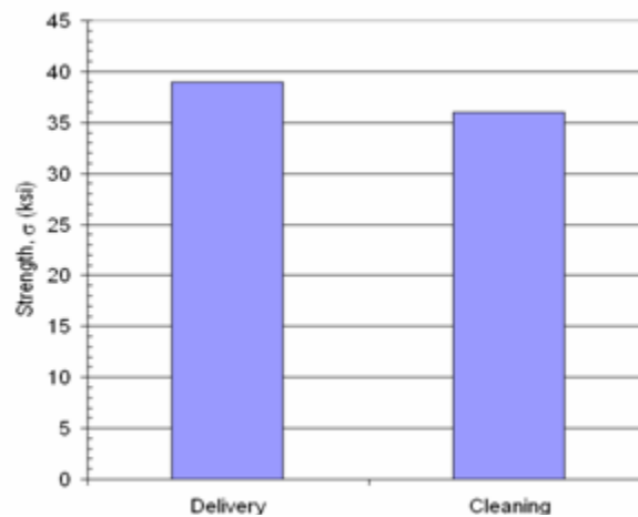
Figure 2.18: Glass Strength Comparison between Deliveries and Cleaning [16]
