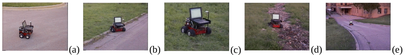
Figure 6: Sequence of images from the building approach mission; (a) the robot is moving out from the parking lot; (b) the robot is crossing over a curb; (c), (d) the robot is navigating a grass and rubble area; (e) the robot is approaching the final destination.
