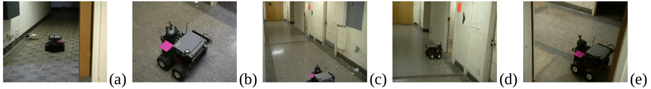
Figure 8: Sequence of images from the indoor assessment Phase II mission; (a) the robot is aligning with the corridor; (b) the robot is navigating the corridor; (c) the robot is recognizing the biohazard sign; (d) the robot is entering the target room; (e) the robot is in the target room.
