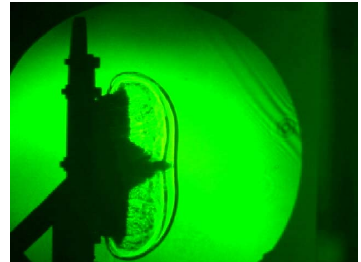
10-cm Lightcraft Shadowgraph Test
