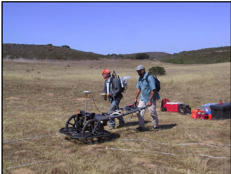
Figure 3.5: Photograph of DNT survey operation underway at the Fort Ord ODDS site. The photograph shows the lane markers at 2-m intervals. For reference, the width of the transmitter antenna is 1 m.
