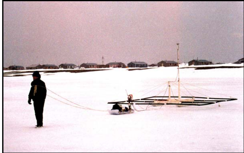
Figure 2.2: Photograph of the sled-mounted DNT antenna system deployed in Gambell, Alaska (St. Lawrence Island) in 2000. The targets were discarded ammunition and other metal objects dumped in a 20-ft deep lake.
