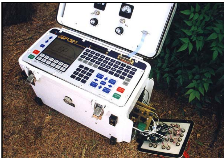
Figure 2.7: Photograph of GDP-32 II multi-function receiver as configured for DNT data acquisition. The side access panel has been removed to expose the NT-32 circuit boards that comprise the imbedded NanoTEM transmitter.
