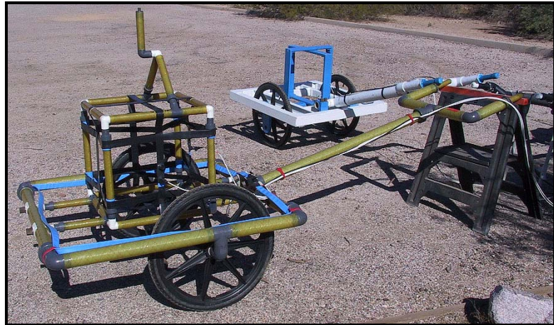
Figure 2.6: Photograph showing two recent versions of cart-mounted DNT antenna arrays. The cart in the foreground is assembled from lightweight fiberglass tubing and weighs only 47 lbs. The cart in the background is manufactured from fiberglass channel beams. It weighs more than 80 lbs.
