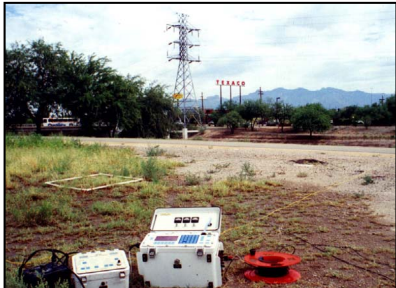
Figure 1.1: An early deployment of NanoTEM for an environmental survey in Tucson, AZ. The system as shown uses a 20-m fixed-loop transmitter and a 1-m roving receiver loop (above the instruments).
