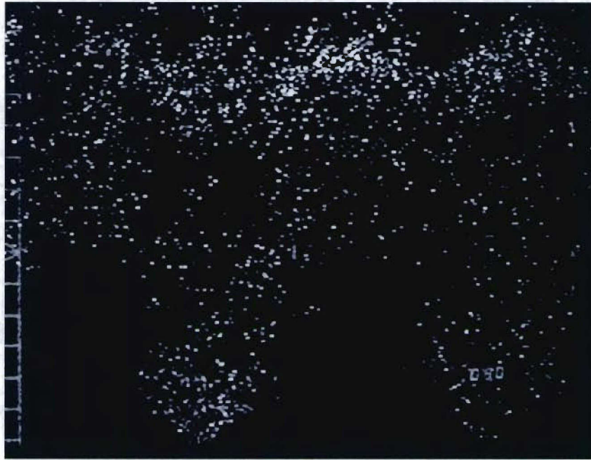
Figure 4. Photograph of the laboratory test section from the side of the tank after the passage of the wing. Nearly neutrally buoyant particles were placed near the top of this photo, in the path of the wing. The vortices, generated by the passage of a lifting wing, picked up the particles and carried them downwards, towards the floor of the tank. This photograph shows the region of two-dimensional flow, in the top half of the tank, where the particles are uniformly distributed, as well as three-dimensional vortex rings, in the bottom half of the tank.
