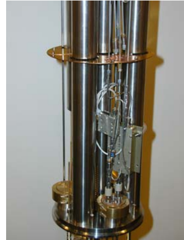
Figure 11: a) Installation at Yale in PI's lab of a new type of dilution refrigerator specially designed for RF experiments. b) Detail of microwave cabling in installation phase. Cryogenic microwave HEMT amplifier is shielded in aluminum box above 4K flange shown at the bottom of picture.
