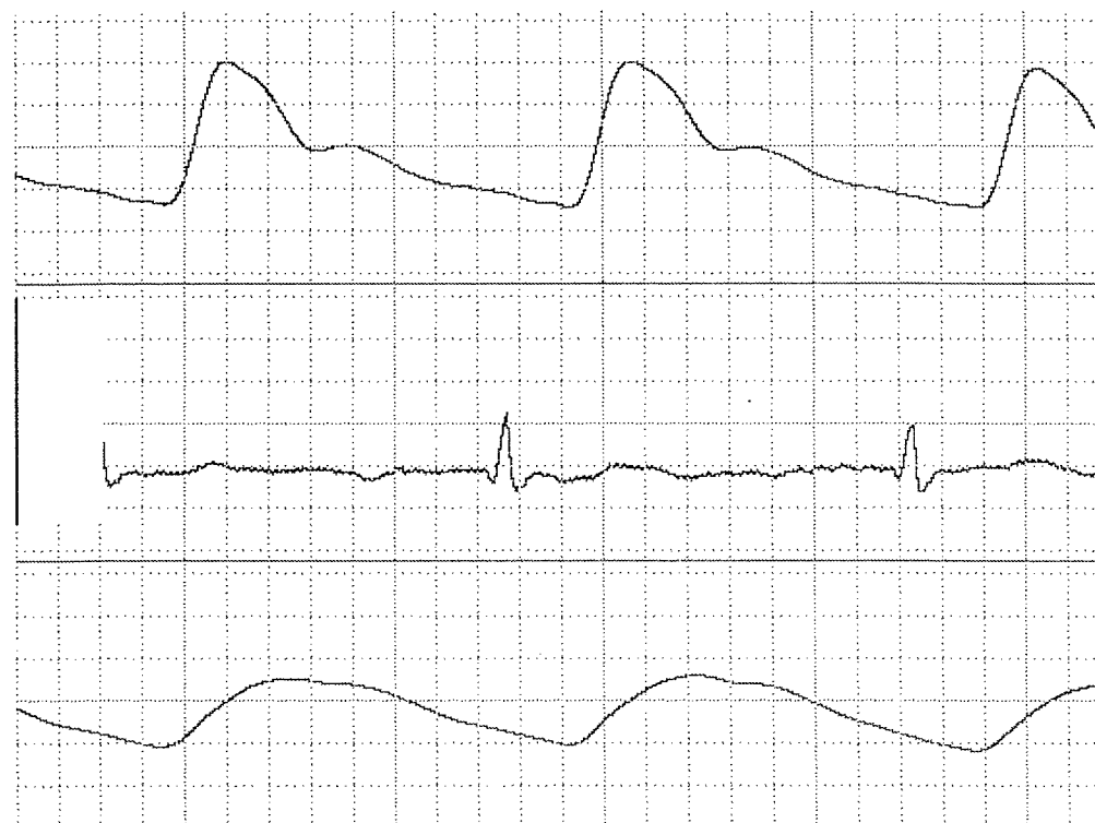
Figure F3. Finger blood pressure (top), EKG (middle), and forearm IPG \Delta R (bottom) traces at 40 mmHg cuff inflation pressure.
