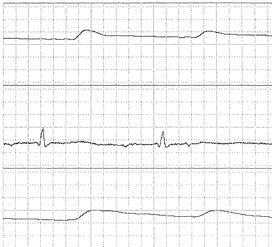
Figure F7. Finger blood pressure (top), EKG (middle), and forearm IPG \Delta R (bottom) traces at 120 mmHg cuff inflation pressure.
