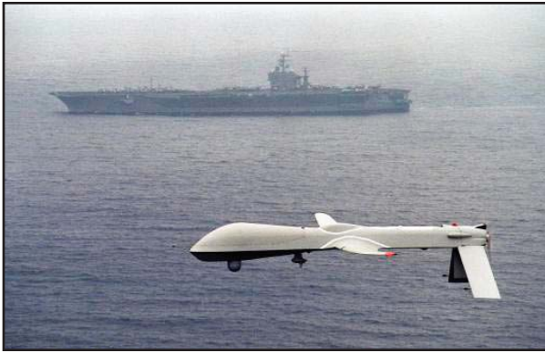
The Predator Unmanned Aerial Vehicle flies down the port side of the USS Carl Vinson. The flight was the Predator's first maritime mission with a carrier battle group and provided near-real-time infrared and color video images of the ship.
