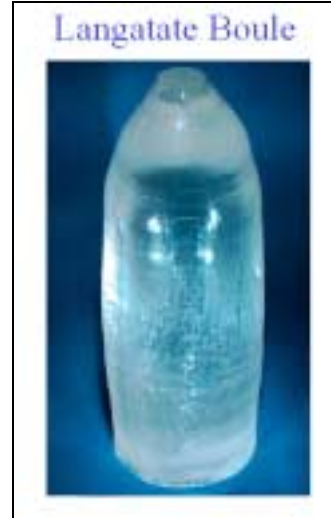
Figure 9. Langatate Boule Developed at Crystal Photonics Inc. by ARL/CECOM for Acceleration-Insensitive Clocks
