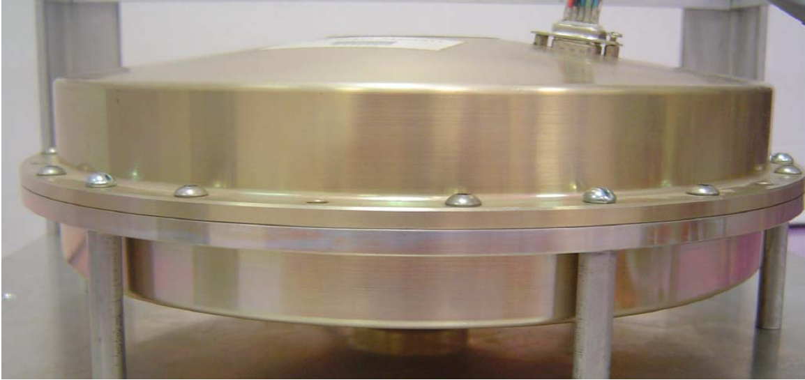
Figure 7. 20.3 N.m.s Reaction Wheel on board AUDASS II
