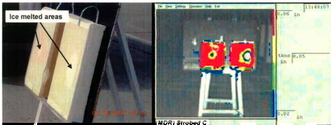
Figure 16: Photo (left) 2B & 3B milled samples with melting, corresponding MDA image (right)
