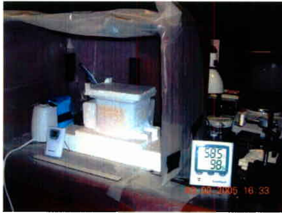
Figure 6: Environmental chamber setup
