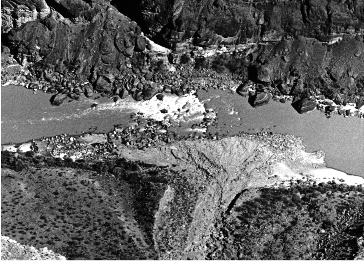
Figure 24. Oblique aerial view of Lava Falls Rapid and Prospect Canyon (May 20, 1964; P. T. Reilly). At a discharge of 37 \text{ m}^3/\text{s} , the 1963 debris-flow deposit constricts the river by about 60 percent; the debris fan initially extended nearly to the middle of the Ledge Hole. This view shows the reworking by a peak discharge of 540 \text{ m}^3/\text{s} . The Meteor Rock is visible in the center of the rapid, and the typically submerged Deflector Rock divided the tail waves.
