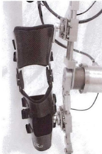
Figure 3: Picture of knee brace and attachment to exoskeleton frame. There are two attachment points between the brace and the exoskeleton frame, one at the thigh, and one at the shank. At each point, there is a quick connect ball joint for easy donning and doffing.
