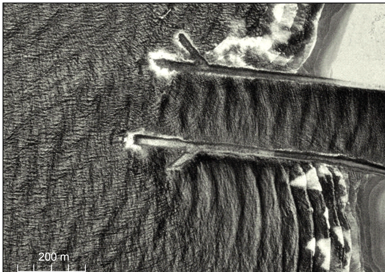
Figure 1. Example of jetty spurs at Siuslaw River Inlet, OR. Spur lengths are 122 m
