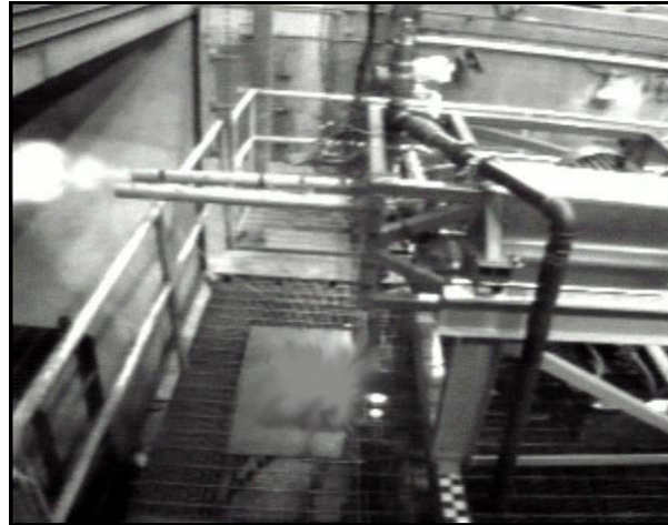
Figure 6. In-house research 'Quad-4' PDE, success on first attempt, 9 September, 1999: 91 second operation at 8Hz, single 2" diameter by 3' long tube, stoichiometric H 2 /air, conventional ignition.
