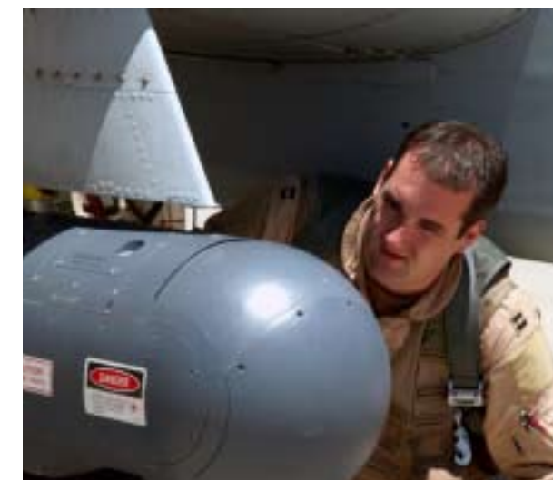
An A-10 pilot checks his Litening Precision Targeting pod before a mission in Afghanistan
