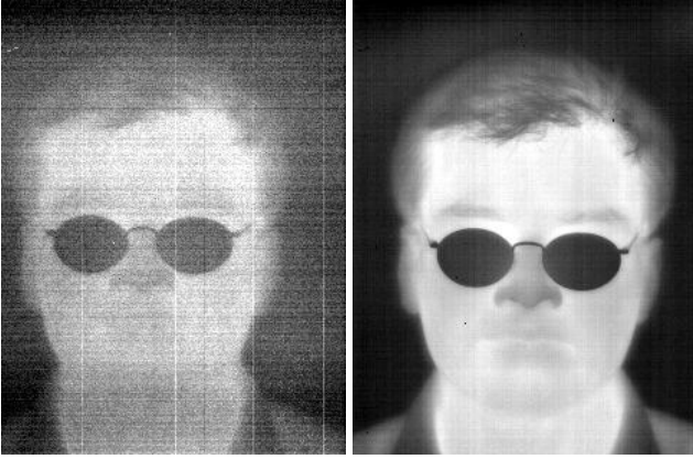
Fig. 1. Uncalibrated (left) and calibrated LWIR images. There is significant pixel-wise non-uniformity in responsivity which is removed by the calibration process.
