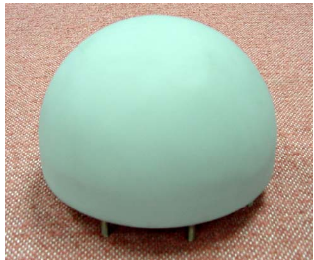
Figure 10 Picture of the new 5.3" 7-element GPS dual-frequency (L1/L2) S-CRPA
