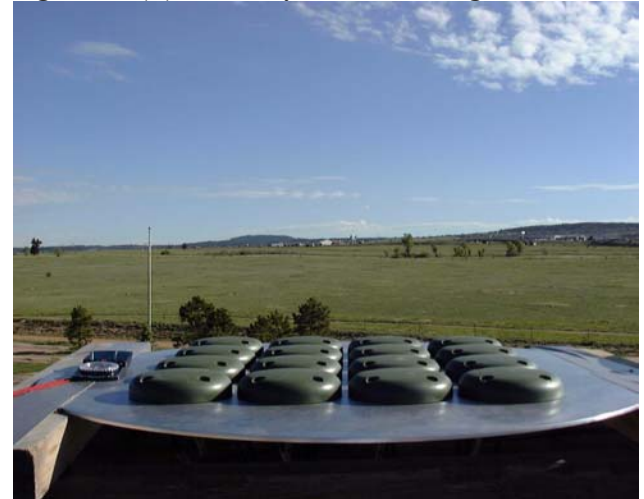
Figure 2 Sixteen Element HAGR Antenna Array
