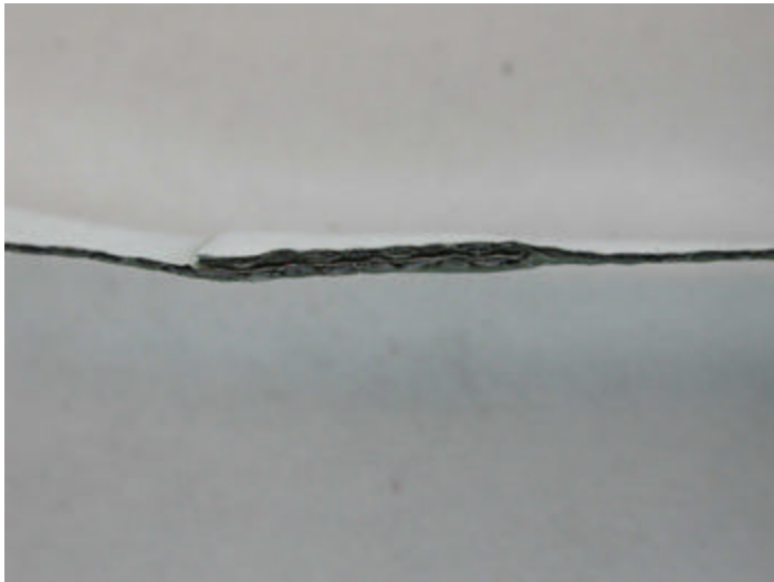
Figure 8 Cross-sectional view of Duraseal™ seam.
