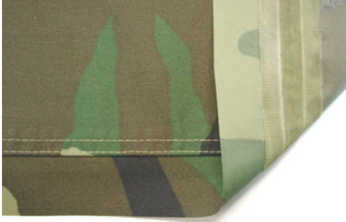
Figure 4 Taping of the sewn seam in a vinyl-coated polyester shelter fabric.
