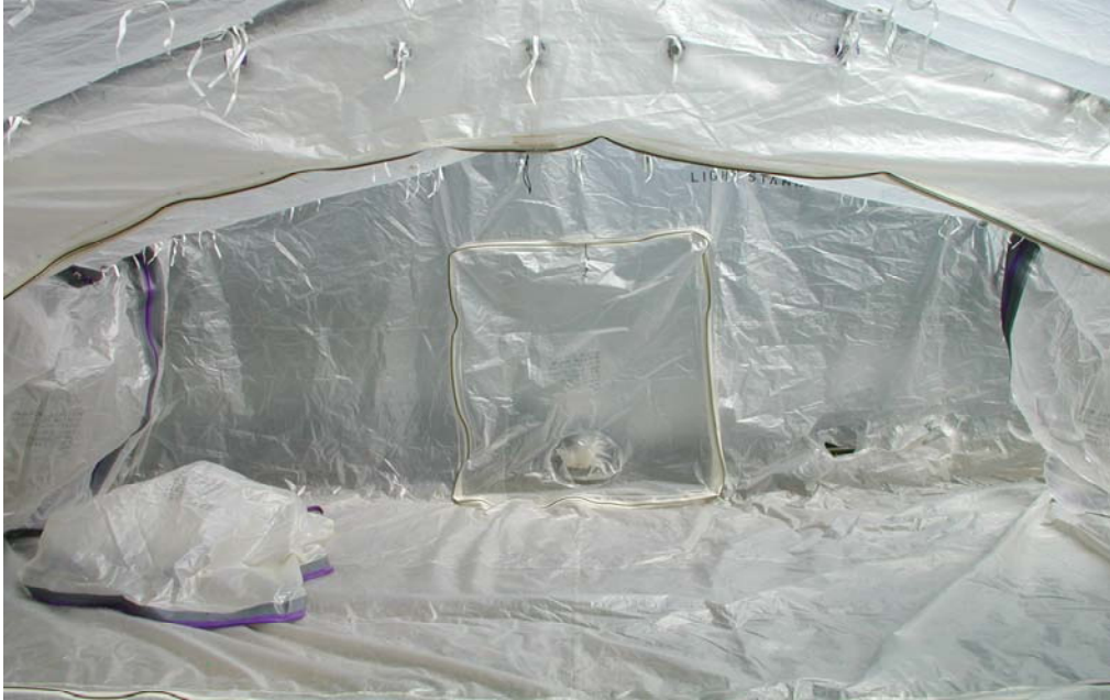
Figure 3. M28 liner: PVDC internal barrier with a HDPE scrim and a LDPE protective coating.
