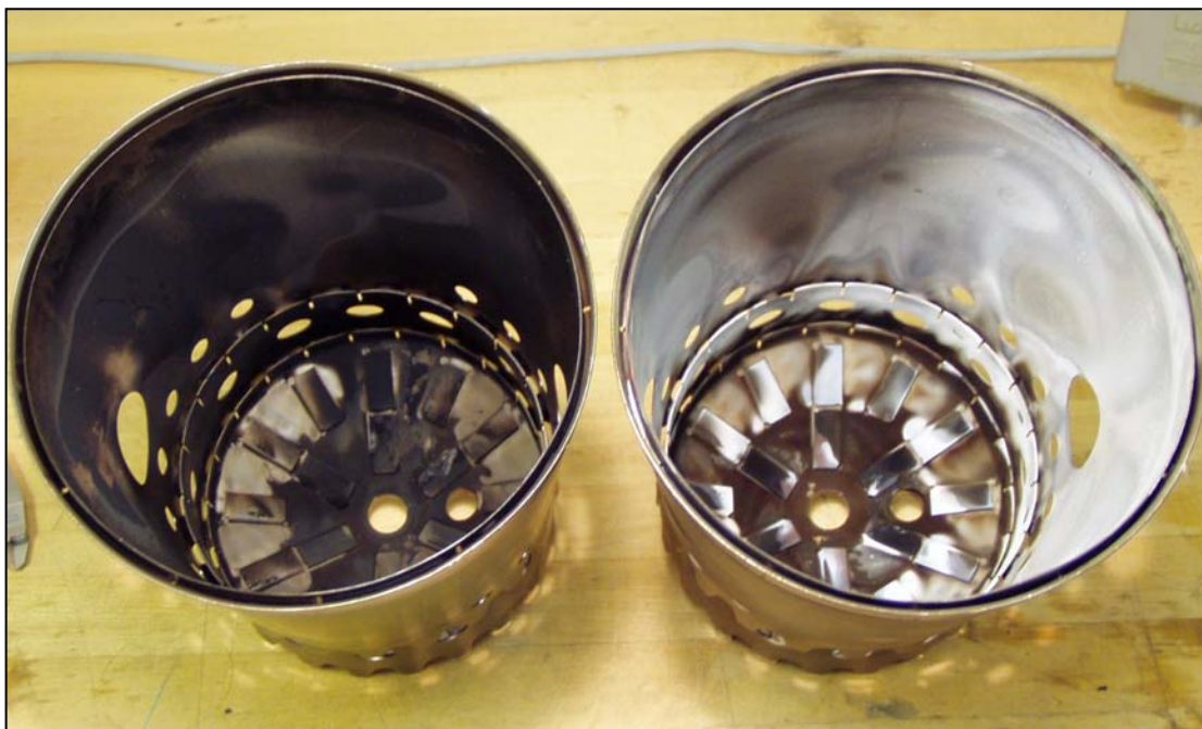
Figure 36. Soot Buildup in two T63 Combustors from a Previous Demonstration Operated 45 hrs on JP-8 and 175 hrs on JP-8+100
