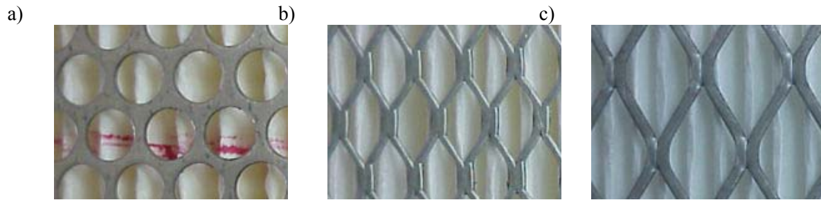
Figure 2. Liner configurations: a) is a perforated metal liner with 0.25” holes and was used only on the filters with Lydall 3255; b) is an expanded metal liner with 0.26” by 0.50” openings and was used for filters with the Lydall 3242 media; c) is an expanded metal liner with 0.47” by 0.80” openings and was used for filters with the Lydall 3282, 4350, and 4450 media.
