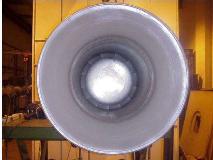
Figure 8. A104 fan installed in test duct with bell-mouth on inlet.
