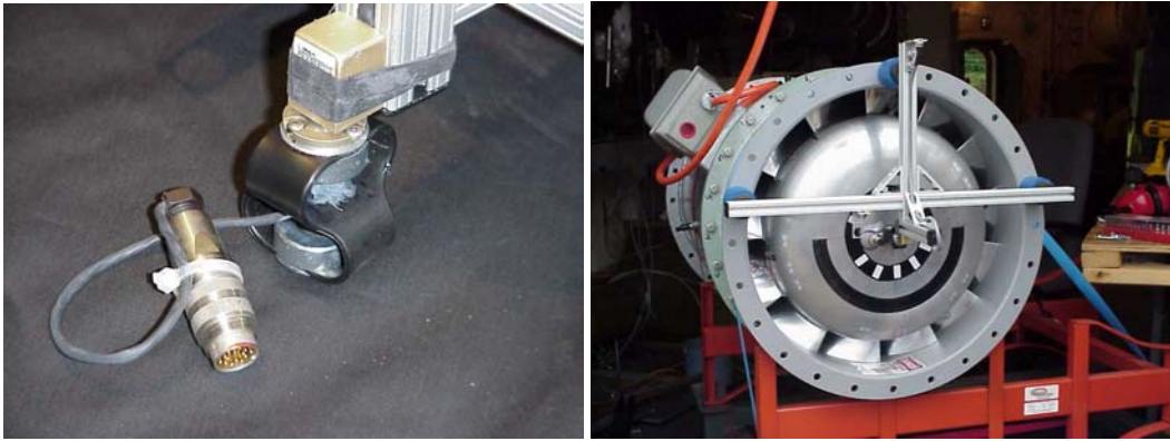
Figure 16. T-rail and 10-conductor slip ring.
