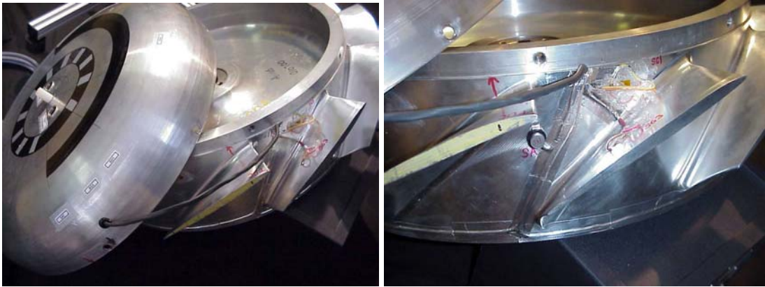
Figure 14. Mounting of shock accelerometer and strain gauges.
