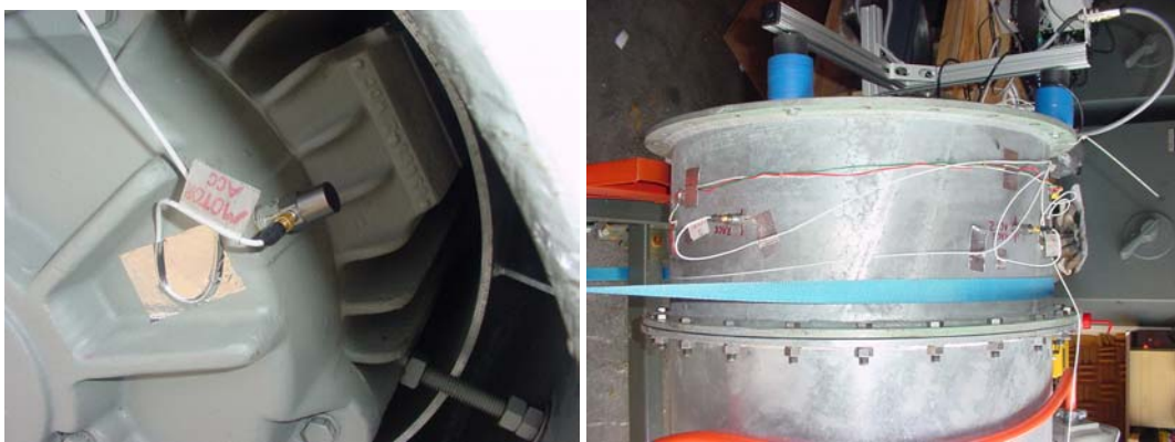
Figure 17. Mounting of motor accelerometer (left) and strain gauge and accelerometers on rotor race (right).
