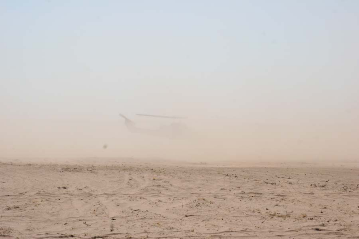
Photo 39. AH-1 landing on untreated helipad
