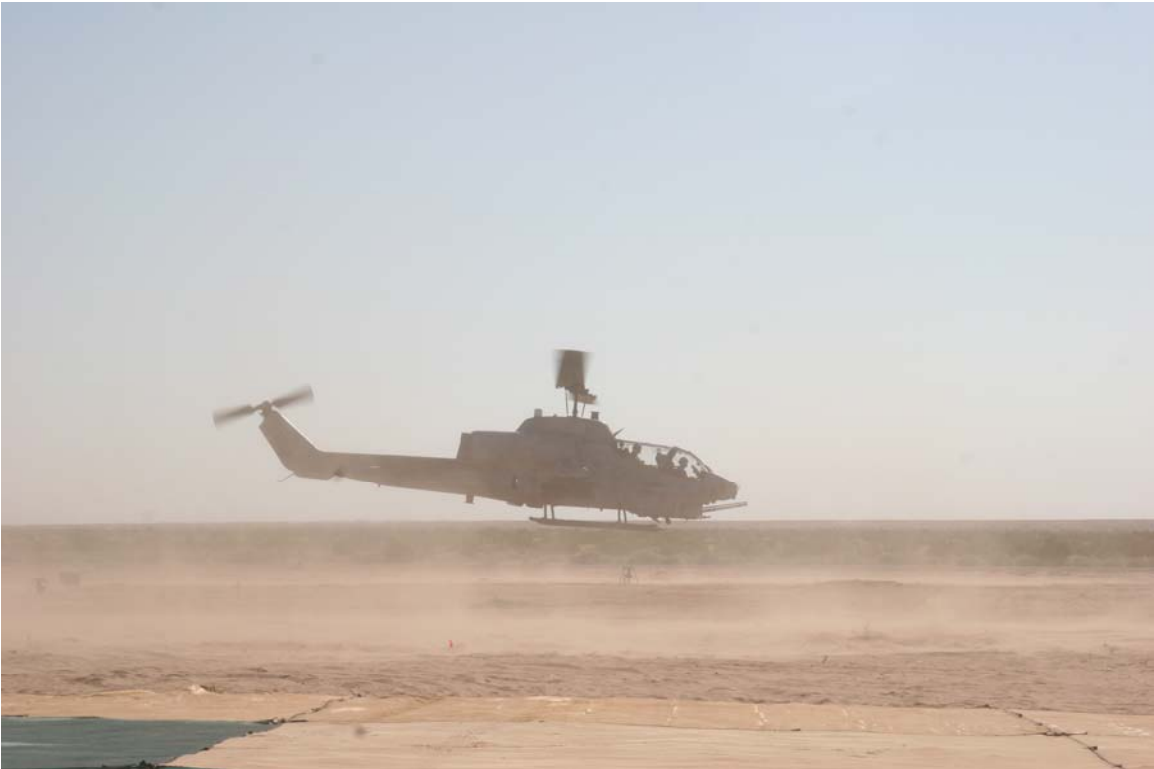
Photo 44. AH-1 landing on helipad 13 (Surtac®, 0.36 gsy)
