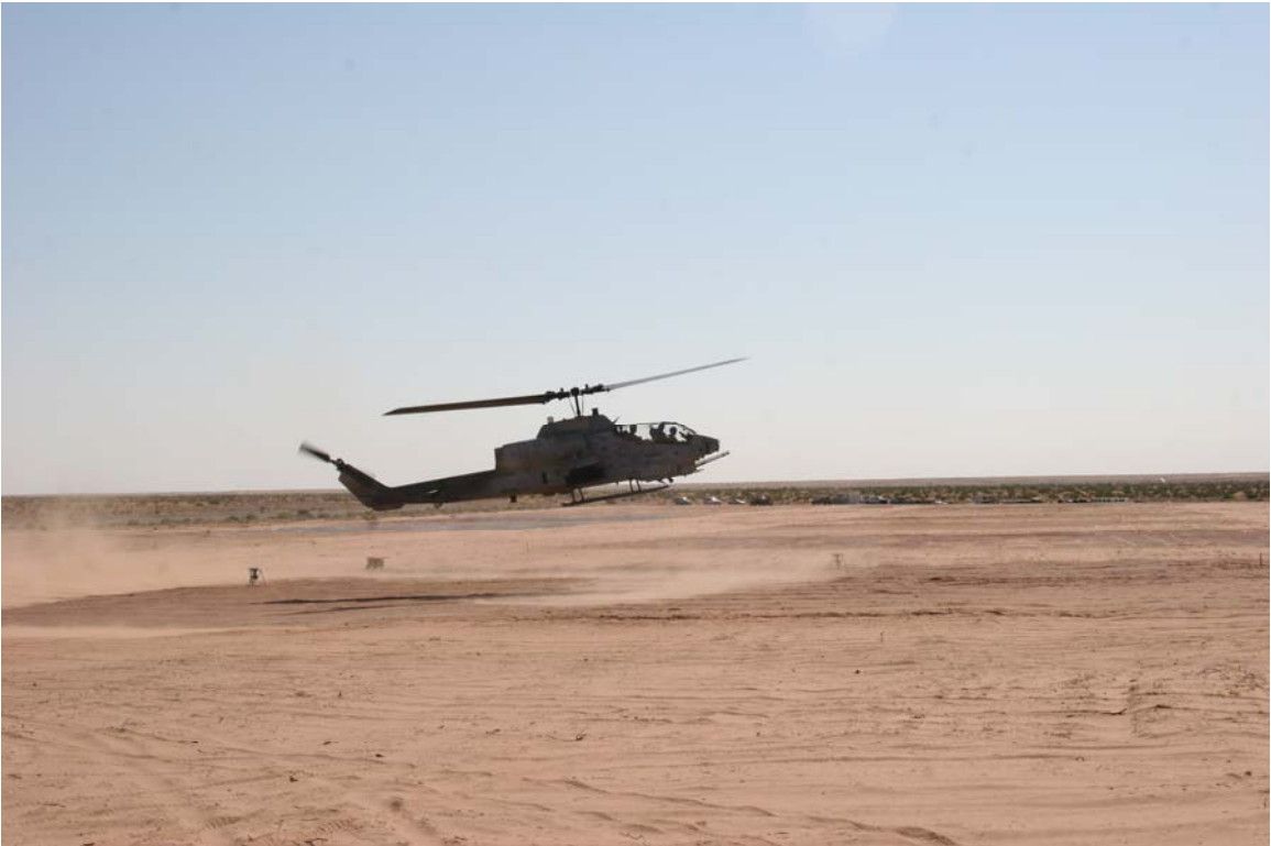
Photo 40. AH-1 landing on helipad 13 (Durasoil®, 0.36 gsy)
