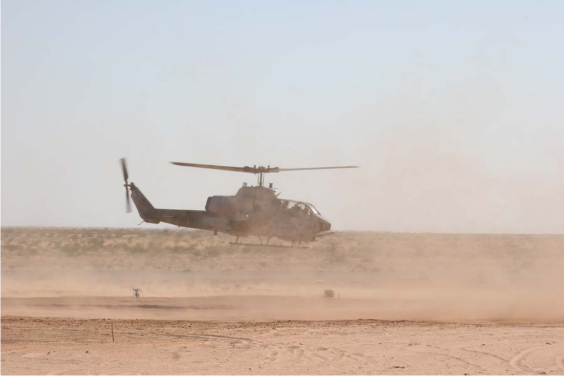
Photo 43. AH-1 landing on helipad 6 (Envirokleen®, 0.6 gsy)
