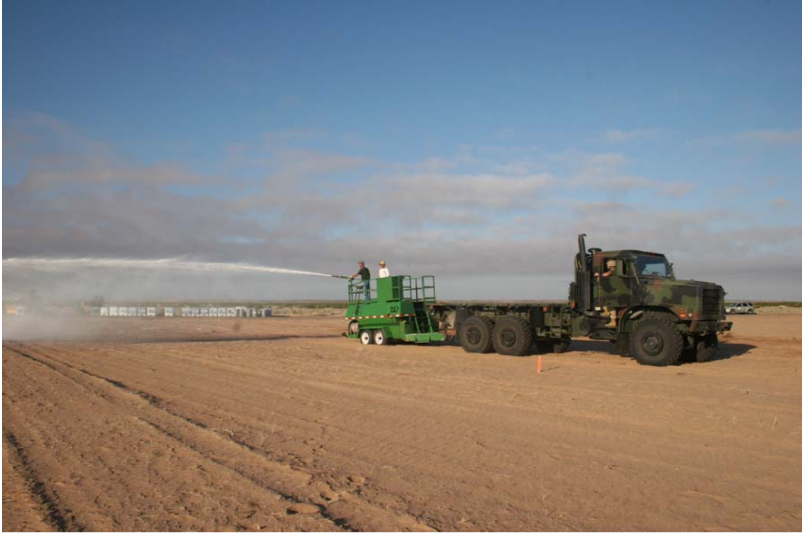
Photo 3. Easy Lawn® C95 trailer-mounted hydroseeder pulled by MTVR
