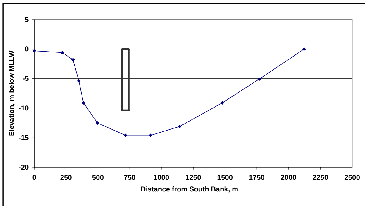
Figure 4. Channel cross section at Pickleweed Trail with 51-m beam by 10.4-m draft ship
