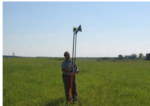
(b) Trihedral retroreflectors in far field of radar.
