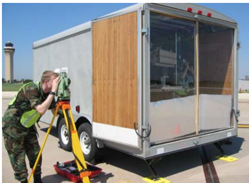
(a) Laser rangefinder total station used to measure distance to calibration targets.
