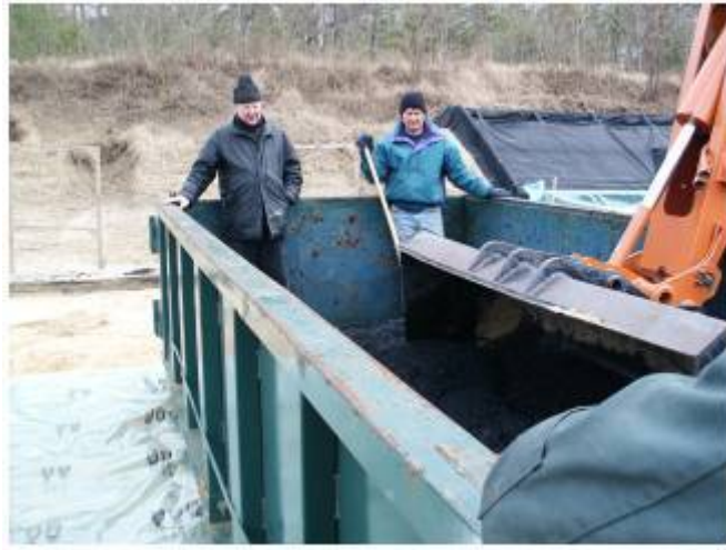
Figure 21. Scooping Loosened Granular Rubber from Roll-off Container.
