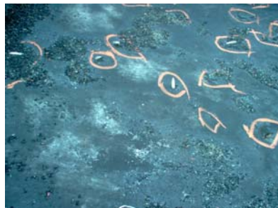
Figures 53, 54 and 55. Holes/Tears (circled) in Bottom Rubber Liner of the Range 5 Bullet Catcher.
