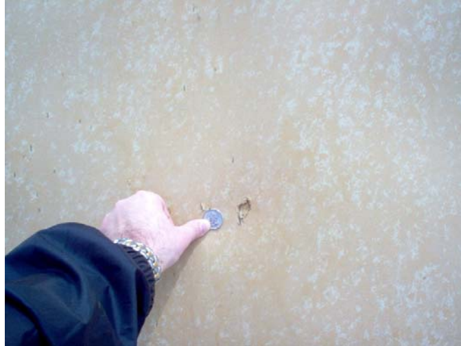
Figure 33. Tear in Top Rubber Cover, Approximately the Size of a U.S. Quarter.
