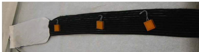
Figure 3: Arrangement of Sensors on Strap
